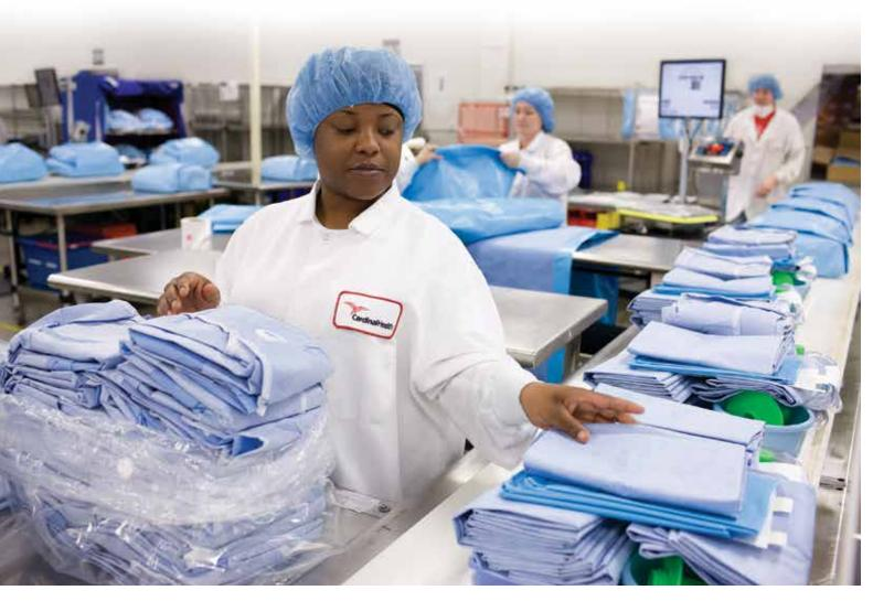
Once we build the surgical kits in our manufacturing area, we put them in a highly specialized plastic bag with Tyvek vents, we seal the bag, and they go through an ethylene oxide sterilization process. When they finish the sterilization process, they are shipped to a cross-dock facility where we consolidate freight, and then we send them to the distribution centers that support the hospitals.
